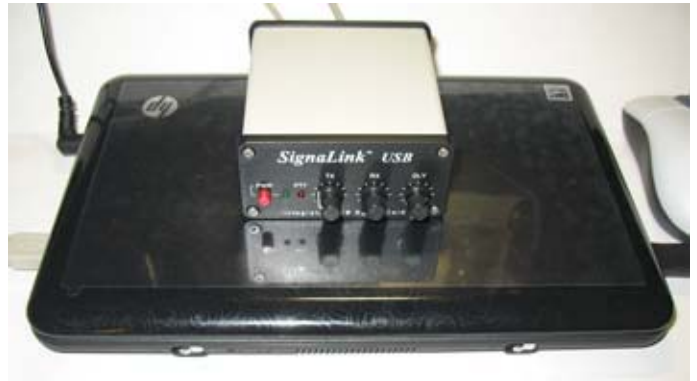
The Signalink USB combined with a small, netbook computer makes a light combination for digital mode operation. Total weight — just 3 lbs.
