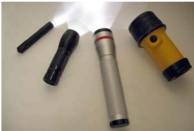
Next-generation LED flashlights use a single high-power white-light LED and produce bright illumination with long battery life. Left-to-right, “Coast” (one AAA battery), “Police” (three AAA), Victorinox (two C cells) and yellow Dorcy light (four AA cells).
