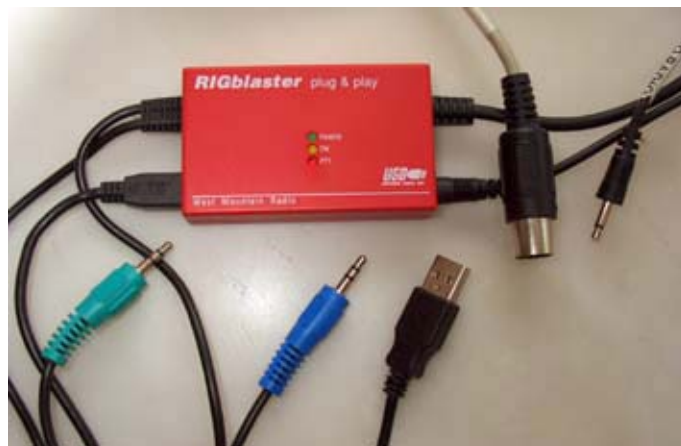
The RIGblaster “plug & play” sound card interface has lots of connectors for (L-to R) PC output audio, PC input audio, USB, transceiver data and transceiver control.
