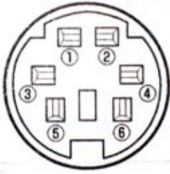
IC-706MkIIG 6-pin mini-DIN Data socket, rear panel view.
